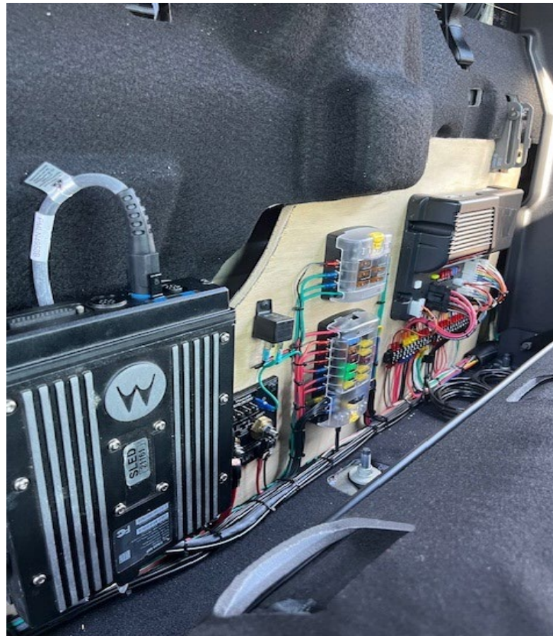
Arson Squad vehicle radio and siren system controls.
